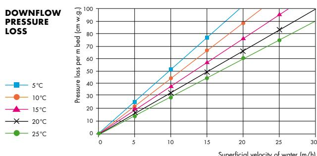
Bed expansion and pressure loss curves are provided for the most commonly used particle sizes. Charts are available for all particle sizes on request.
